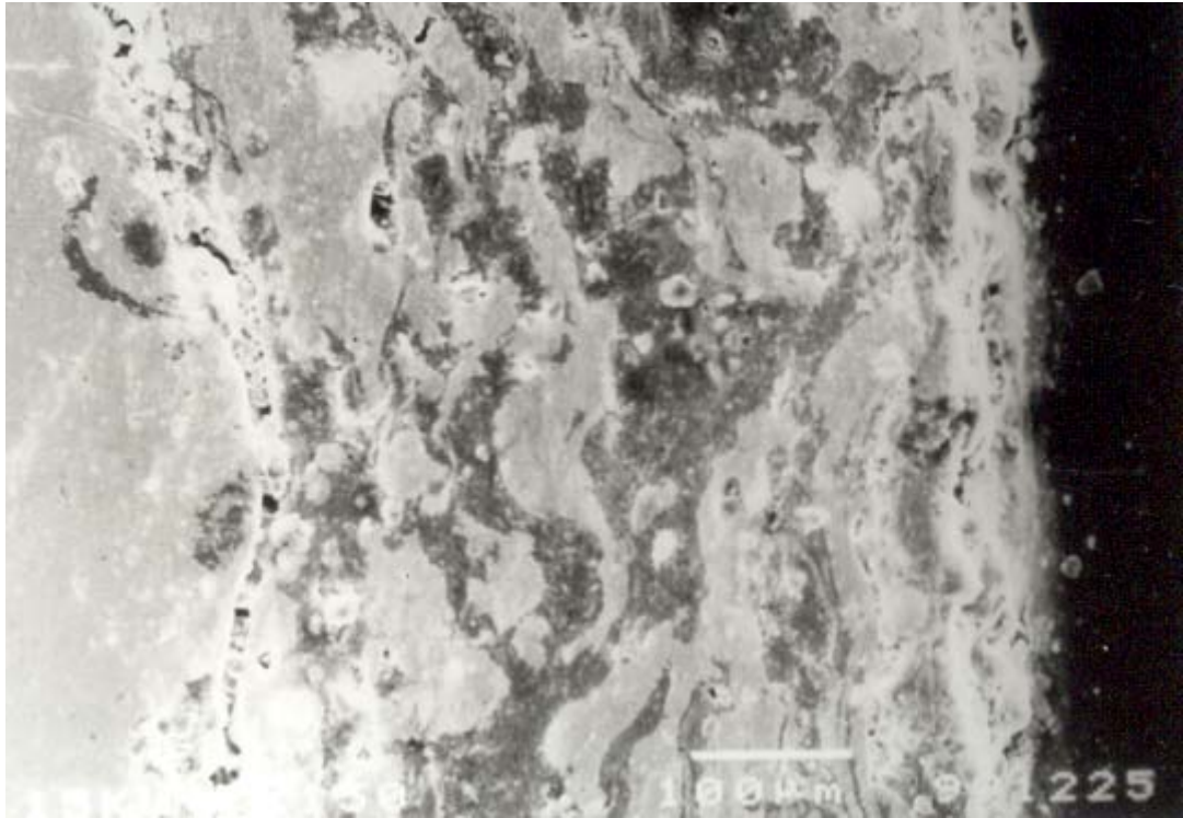
Fig. 4.20(a) Coating interface of (alumina) over Ni+Al bond coat on Copper Substrate.
