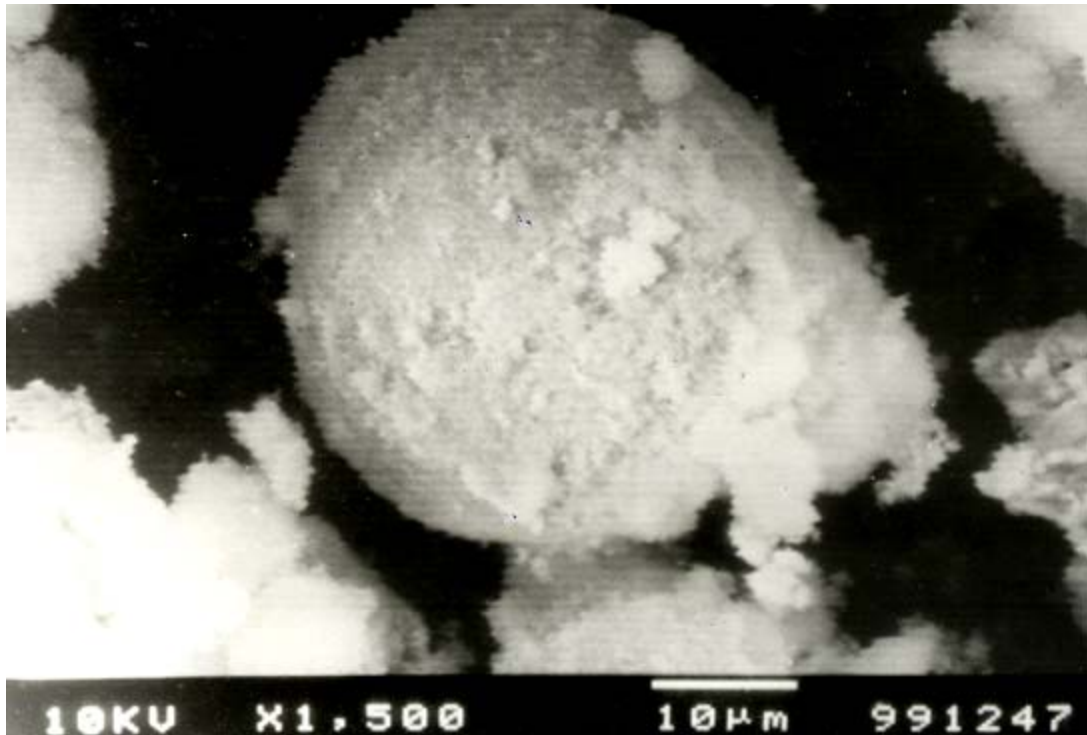
Fig. 4.17(d) Surface morphology (SEM micrograph) of Ni-Al spheroidised powders, processed at 10kW power level, 100mm TBD but with higher magnification(x1, 500).
