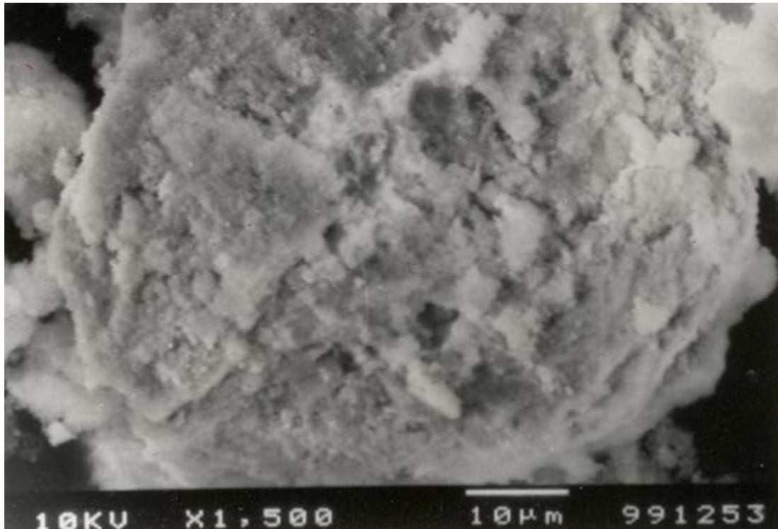
Fig. 4.17(f) Surface morphology (SEM micrograph) of Ni-Al spheroidised powders, processed at 16kW power level, 400mm TBD but with higher magnification(x1, 500).
