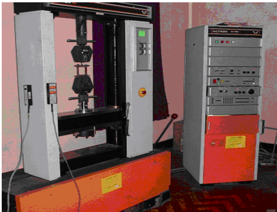
Fig.3.6 Adhesion test set up Instron 1195
