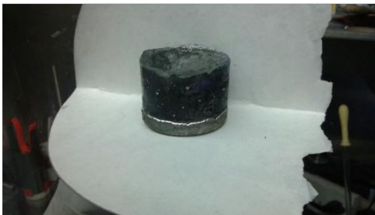
Figure 5.5. Photograph of the \text{LiF}-\text{ThF}_4/\text{Bi-Li} ingot. Note the salt color difference when compared with Figure 5.3.
