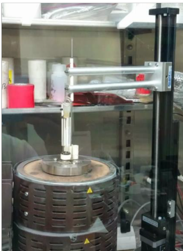
Figure 11.6. Photograph of the vertical translator (Velmex XN10-0012-M02-71) with aluminum arms for holding the WE.
