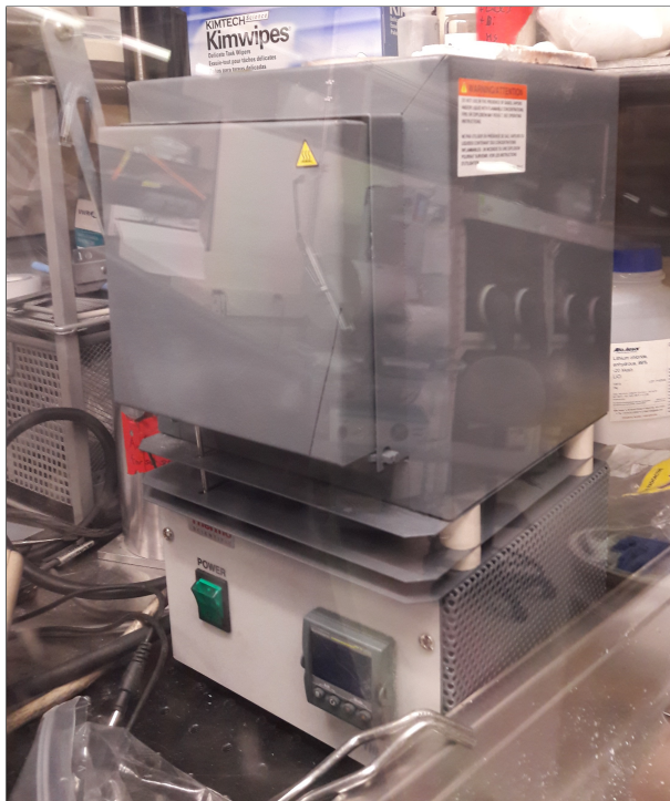
Figure 11.1. Photograph of the furnace (Thermo Scientific Thermolyne) used in later runs.
