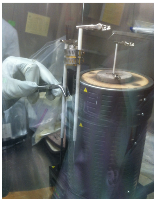
Figure 5.2. Photograph of the electrochemical setup showing the furnace (Kerr Auto Electro-Melt) with alumina lid and the three-electrode setup (WE and CE held together by a nut and a hose clamp, RE sitting independently in the lid).
