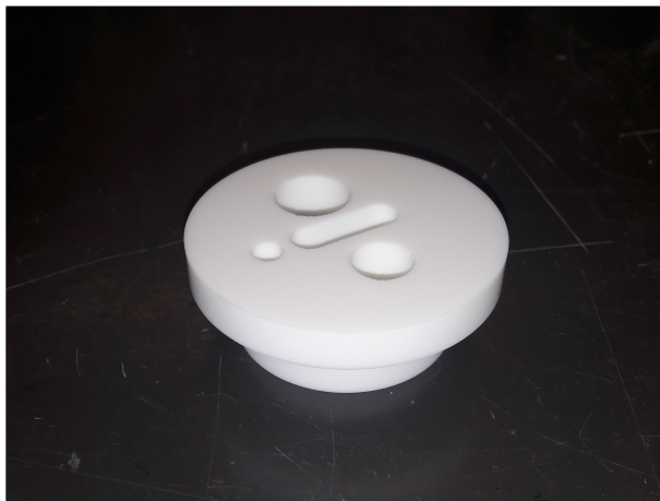
Figure 11.2. Photograph of the macor custom manufactured lid.
