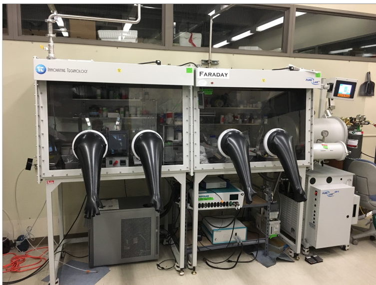
Figure 5.1. Photograph of the inert atmosphere glovebox, potentiostat and chiller setup.
