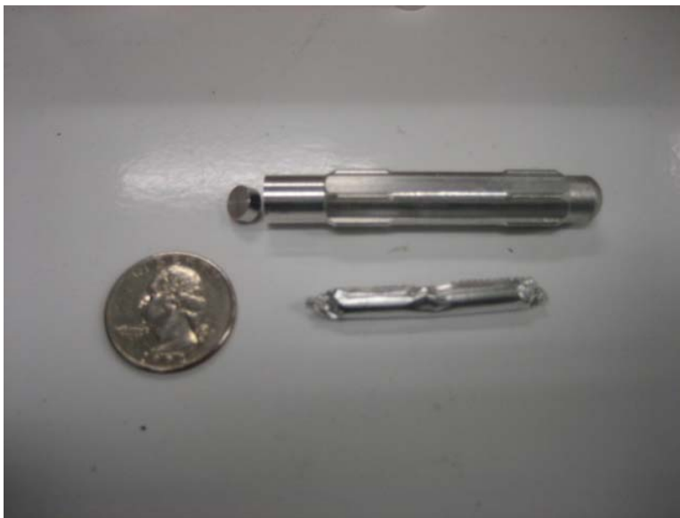
Figure 3.2: Quartz Ampoules in Aluminum Foil
