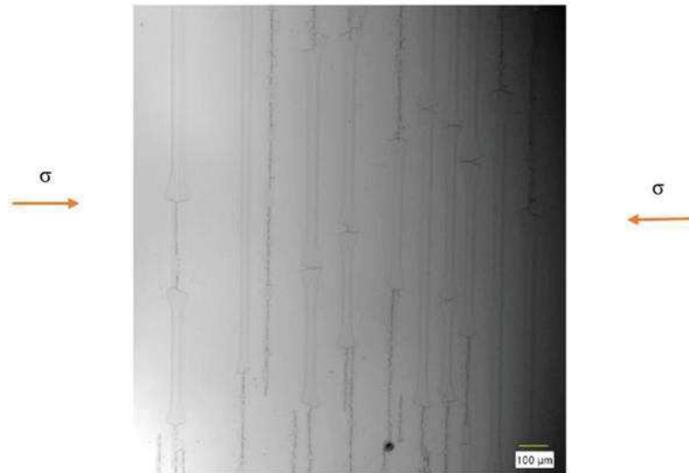
FIG. 6. Optical Microscope observation of buckles and cracks after micro-compression tests. Concomitance of buckles and cracks (x 5). Buckles and transverse cracks (x 20).
