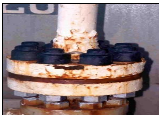
Fig. 4 Crevice corrosion in the junction of pipelines (CTL, 2010)
