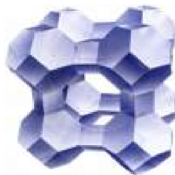
Figure2.10 type A zeolite ‘unit cell’
