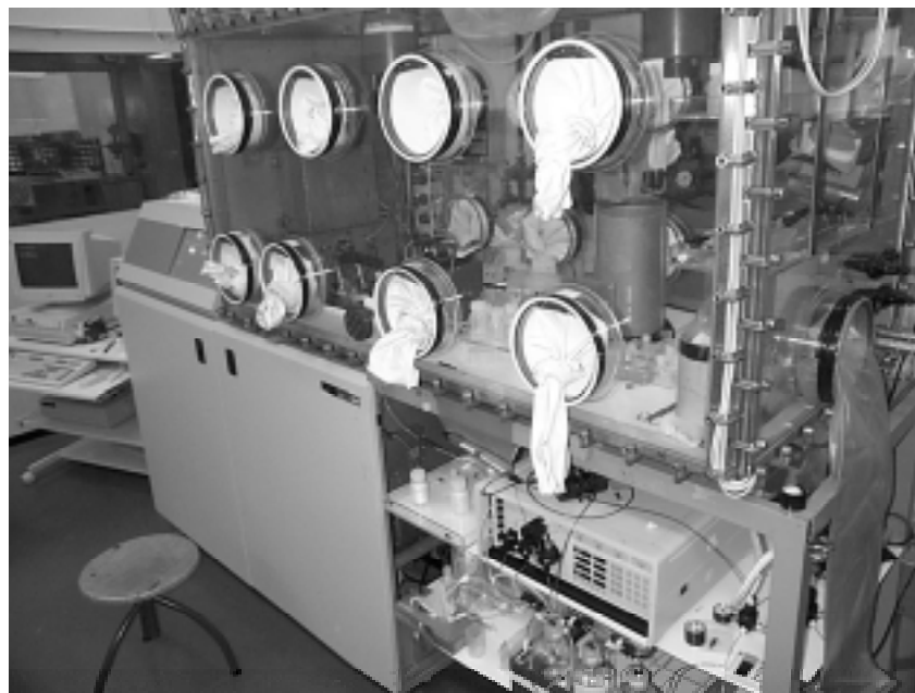
Figure 8. A glove box ICP-MS system installed in the hot laboratory. The HPLC pump can be seen under the glove-box.
