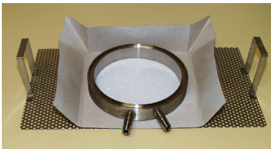
Figure 3. Experimental set-up for migration test using Tenax at high temperature. The migration collar outlines an exact area of 1 dm 2 , which is covered by the Tenax. The steel rack makes sample handling easier.
