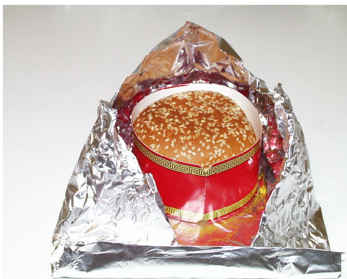
Figure 4. Experimental set-up for migration test with roll. The hamburger collar was put around the roll and this was wrapped in aluminum foil.
