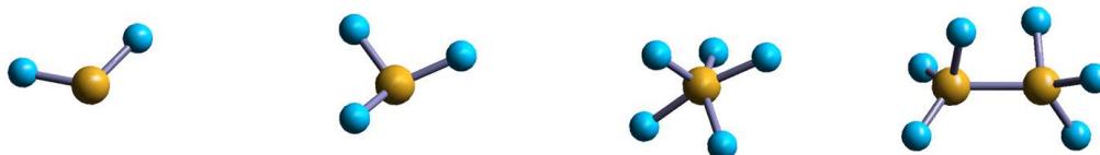
Figure 5.12: Silicon defects in the amorphous silicon-nitrogen alloys. (far left) 2-fold coordinated Si, (left) 3-fold coordinated Si, more specifically a K center, (right) 5-fold coordinated Si, (far right) a Si-Si unit or Si cluster with one Si-Si bond.
