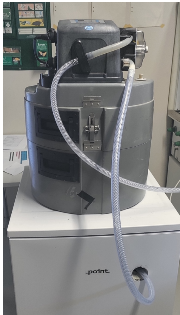
Figure 6. The HACH AS950 composite sampler pumped grab samples to the sample container placed in the refrigerator to obtain a composite sample from one day.
