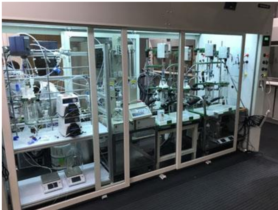
Figure 2: Flow process design consisting of a series of five reactors coupled with multiple recirculating temperature controllers, scales and pumps 21
